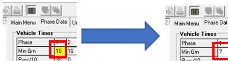
Figure 99: When the Compare mode is active, parameters that are different in the Centrac database will flash yellow to indicate to the user where the difference is. Both the controller and the stored values will be shown.
