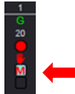
Figure 43: A vehicle asserted call is reflected with the red M in the detector status box under the phase number.
