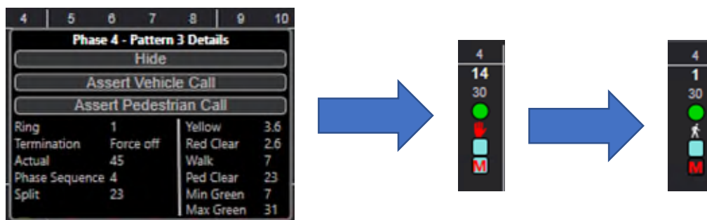
Figure 143: The engineer hovers the mouse over Phase 4 in the Intersection Status Window and asserts a manual pedestrian call to watch pedestrian operations.
