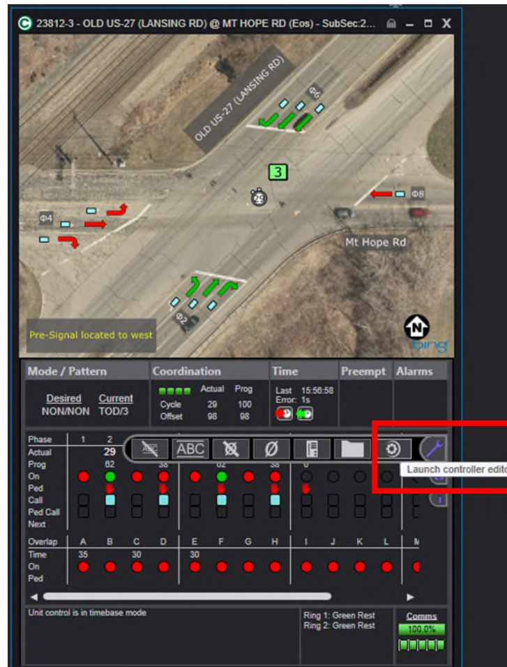
Figure 88: Navigating to the database editor (also known as the controller editor) from the wrench menu in the intersection status screen.
