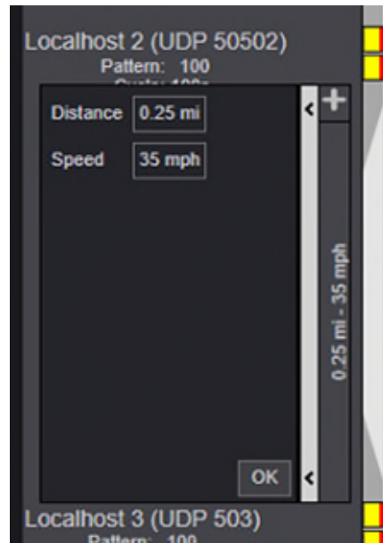
Figure 127: Entering distance and speed data into the expanded link between signals.
