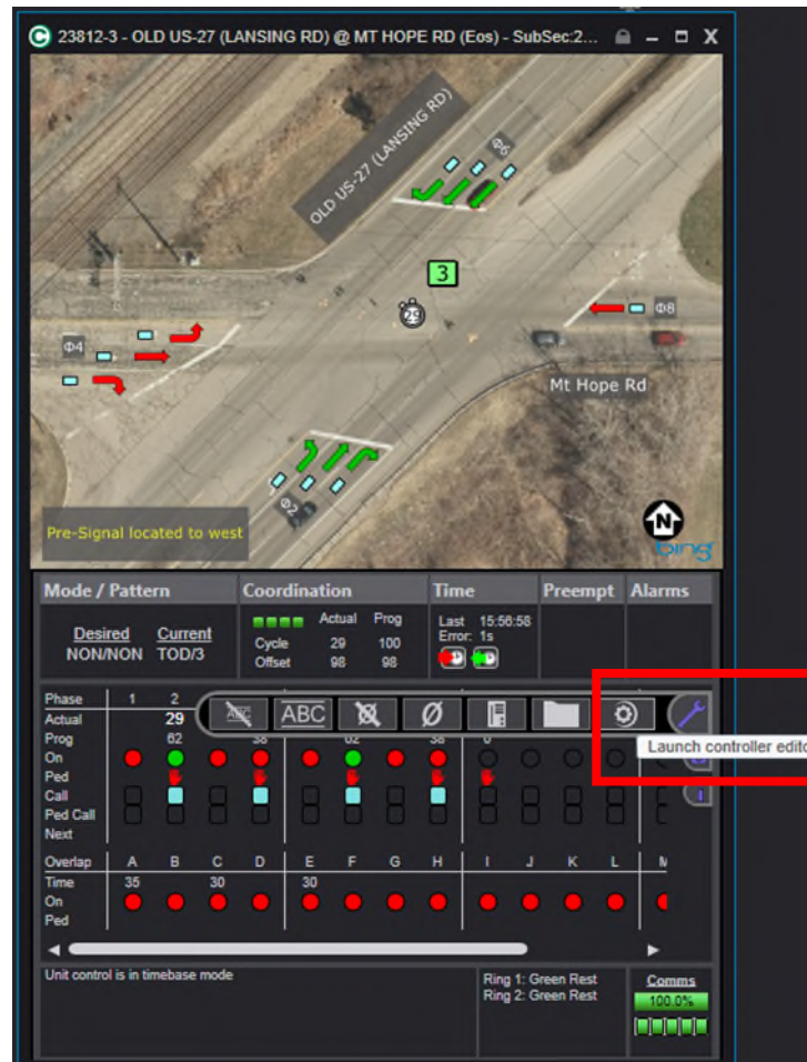
Figure 69: Navigating to the database editor (also known as the controller editor) from the wrench menu in the intersection status screen.
